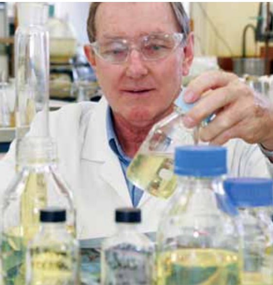
Principal Chemist Fuels Technology Laurie Palmer tests the storage stability of diesel blended with biodiesel in the laboratory at Caltex's Lytton refinery.
